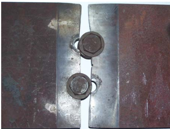
Figure 5. The zone of fatigue fracture of sample with drilled holes and high strength bolts
