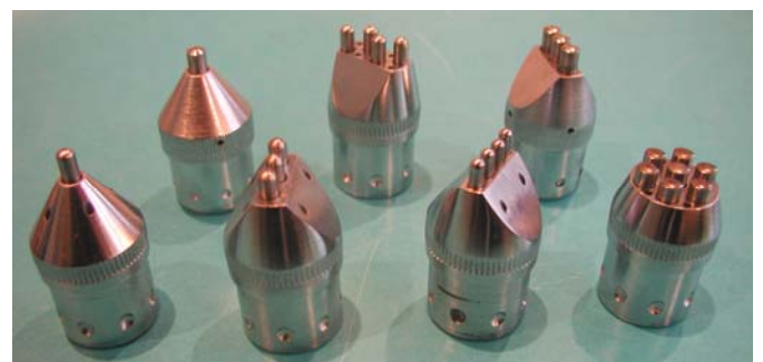
Figure 2. Set of the changeable working heads for different application of Ultrasonic Peening
