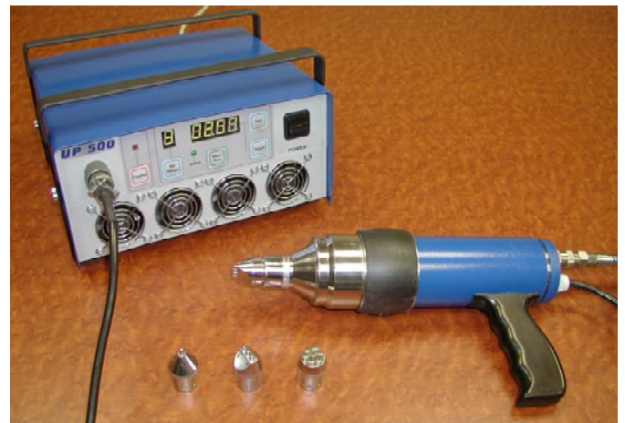
Figure 1. Basic Ultrasonic Peening system for fatigue life improvement of welded elements and structures
