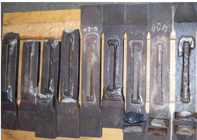
Figure 9. The view of welded samples after repair and subsequent fatigue testing
