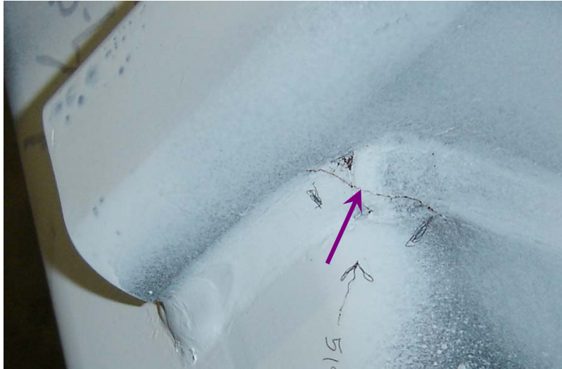
Figure 14. The zone of origination of the fatigue crack (shown by arrow) in the sample that was subjected to fatigue loading after Ultrasonic Peening.
