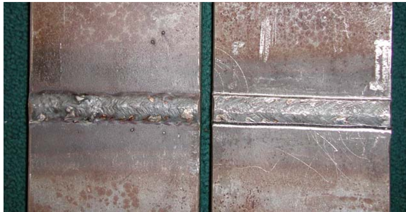
Figure 5. The view of the butt welds in as-welded condition (left side sample) and after application of UP (right side sample)
