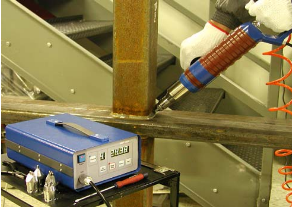
Figure 6. Using of basic UP system for fatigue life improvement of tubular welded joint.
