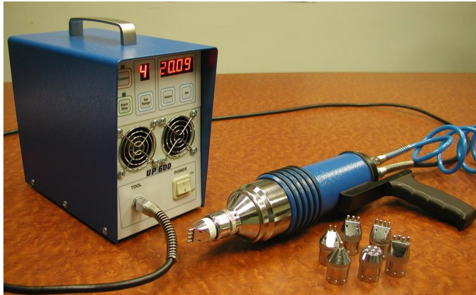
Figure 5. UIT/UP system that is based on using of piezoceramic transducer
