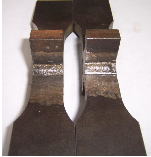
Figure 9. The view of the fillet welds in as-welded condition (left side sample) and after application of UIT/UP (right side sample)
