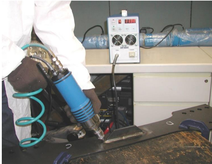
Figure 11. The process of UIT/UP of welded sample for fatigue testing
