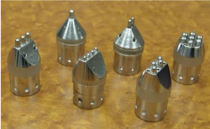
Figure 3. A standard set of interchangeable working heads with freely movable strikers for different applications of UIT/UP [17]
