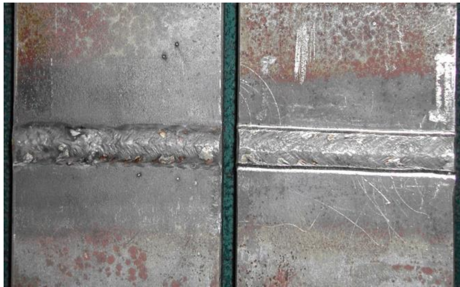
Figure 8. The view of the butt welds in as-welded condition (left side sample) and after application of UIT/UP (right side sample)
