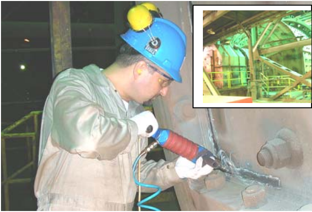
Figure 12. Application of UP for rehabilitation and repair of welded elements of mining equipment
