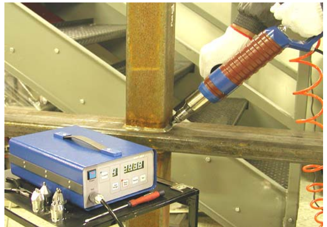
Figure 1. Using of basic UP system for fatigue life improvement of tubular welded joint
