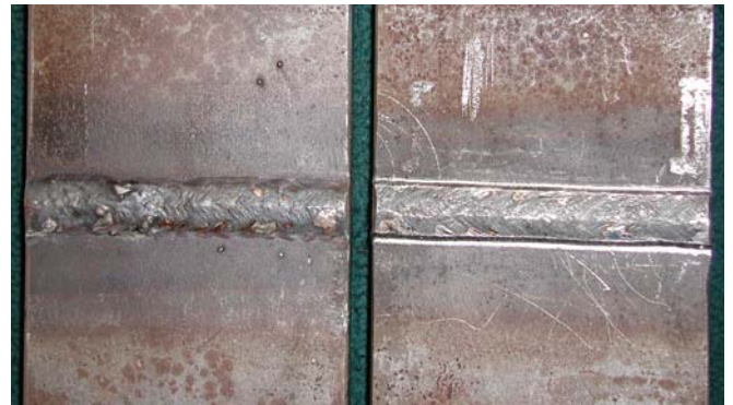
Figure 5. The view of the butt welds in as-welded condition (left side sample) and after application of UP (right side sample)
