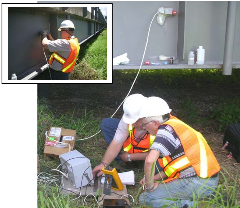
Figure 14. Process of measurement of residual stresses in a welded bridge
