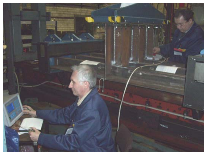
Figure 12. Measurement of residual stresses using UltraMARS system in large-scale welded panel in as-welded condition and during the fatigue loading of the panel
