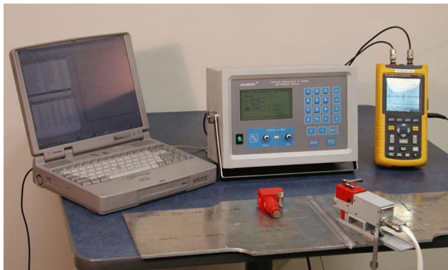
Figure 3. The Ultrasonic Computerized Complex for measurement of residual and applied stresses
