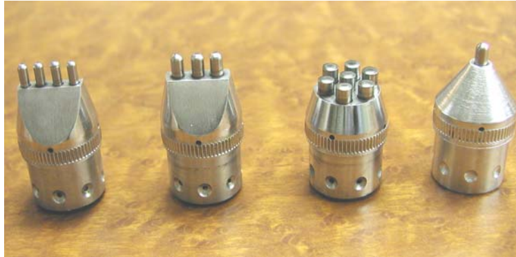
Figure 8. Basic set of the changeable working heads
